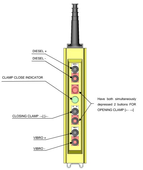
Press the « Close Clamp  $\rightarrow$ ][ $\leftarrow$ » button. This button remains locked. Wait until the green indicator on the button box lights up
